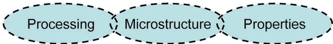
Figure 1-2: The paradigm of materials science. The microstructure of a material depends on the way that it is processed, and the properties depend on the
