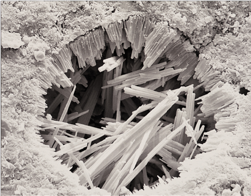
Figure 5-8. Cluster of needle-shaped ettringite crystals deposited in a cement paste void. (Image courtesy of the Portland Cement Association (12494)).
