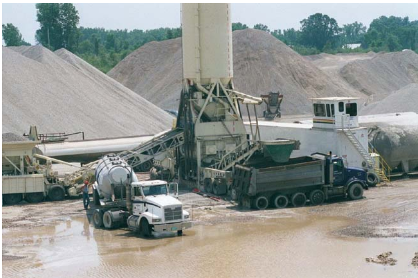
Figure 3-1: Left: A ready-mix plant surrounded by piles of stored aggregate (40-4A). Right: A concrete truck being filled with fresh premixed concrete. (Images courtesy of the Portland Cement Association).
